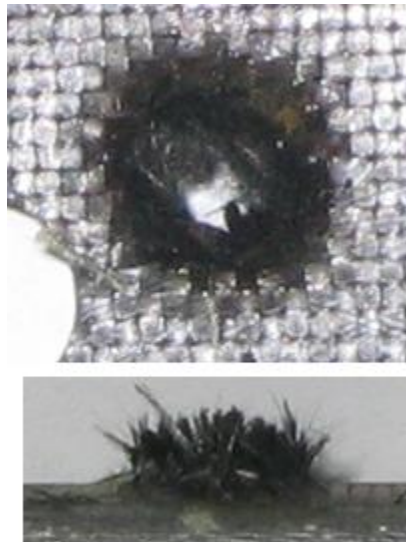
Figure 3.12: Defect during high-feed drilling
