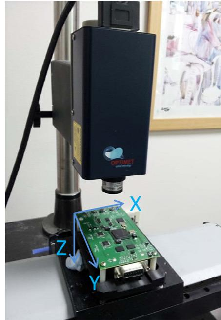
Figure 3 - Optimet's ConoProbe Mark10 HD
